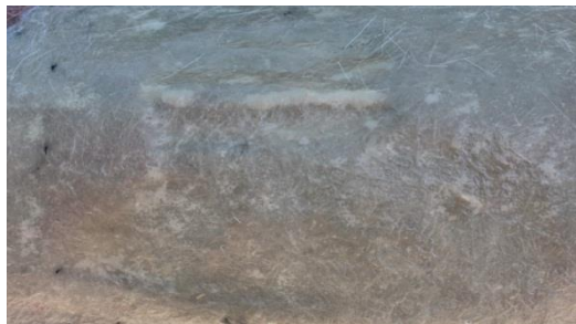
Gambar 8. Hasil tambalan kapal fiberglass
