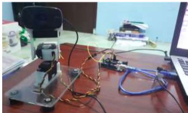
Picture. 3. Pan and Tilt Construction
