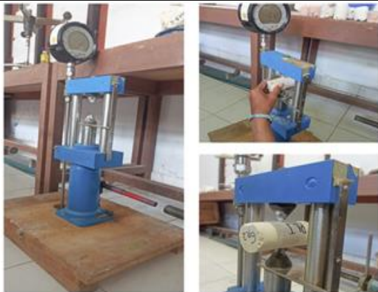
Figure 4. Compressive Strength Testing Using Point Load Machine (Geotechnical Laboratory, Universitas Cenderawasih)
